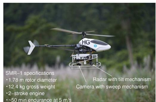
**Figure 1.** CSIRO SMR-1 helicopter configured for weed survey flights over mountainous rainforest.
