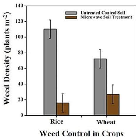
**Figure 2.** Effect of pre-cropping microwave soil heating on the weed density of rice and wheat crop measured at crop harvesting at Dookie, Victoria.
