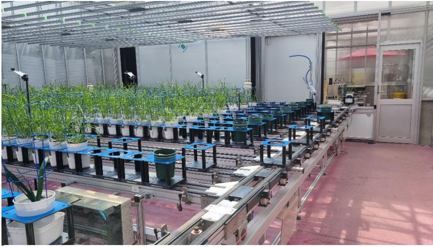
The robotic phenotyping greenhouse at the Australian Plant Phenomics Facility (APPF). The system automatically images, waters, and moves the pots.
